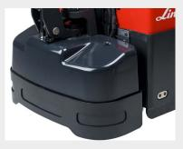
Robust metal cover protects the drive system, also provides safety protection on feet
